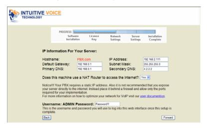
4. In the **Network Settings** window, modify the Default Gateway, Primary DNS, IP Address (static), Subnet Mask, and Secondary DNS as required.
